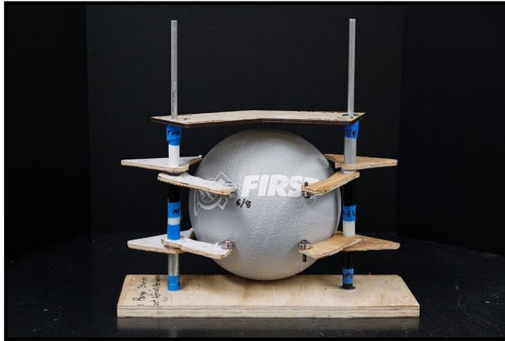
Wooden prototype of pneumatically actuated fingers
