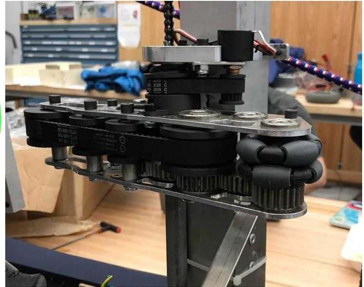
The Flippy Arms were designed to transfer the cargo from the intake into the Catapult. They hold the cargo in place in the catapult as the turret aligns and then open up to release the ball when the catapult fires.
